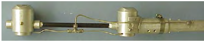
Figure 3. Photograph of one of the measurement tools showing the plumbing for couplant transport and pressurizing the air cylinders. Transducer separation is 30.5 cm (1 ft).
